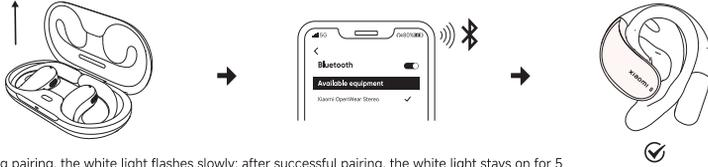
During pairing, the white light flashes slowly; after successful pairing, the white light stays on for 5 seconds then turns off; if there is no device pairing for 1 minute, the indicator light turns off.
