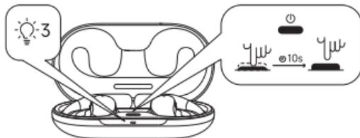
Press and hold for 10 seconds until the orange light flashes three times
