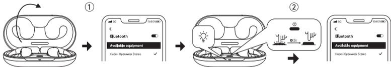
Keep both earbuds in the box, press and hold for 2 seconds until the white light flashes slowly to enter pairing mode, then you can connect to a second device.
